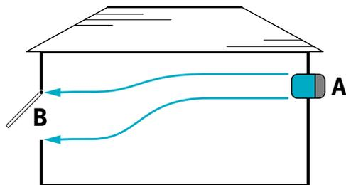
Window or door space at B should be opened to twice the size of air conditioner intake at A.
